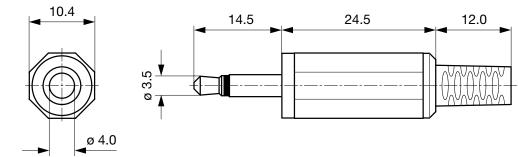
Cable diameter max. 4.0 mm
