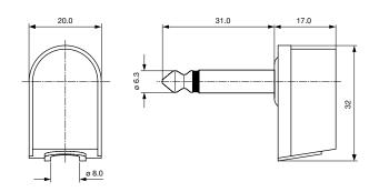
Cable diameter max. 8.0 mm
