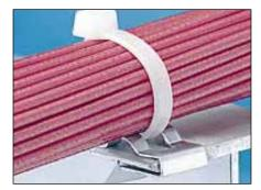
The mount clips on sheet metal edges for fast mounting of harnesses with cable ties. Ties may be inserted from any of the four sides for easy harness orientation.
