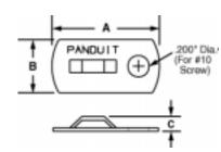
• NOTE: Mount can also be installed with a user supplied adhesive.
