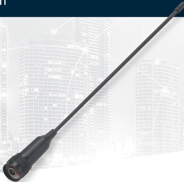
The FW.24 is a flexible 2.4GHz omni-directional whip antenna with an N type (M) connector for outdoor use. It features excellent efficiency (>75%) and high peak gain (>4 dBi) between 2400-2500MHz on a 30x30 cm ground plane.
