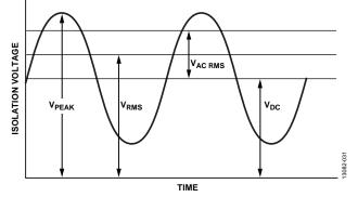
Figure 27. Critical Voltage Example
