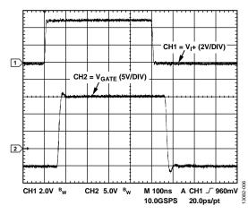
Figure 6. Typical Input to Output Waveform, 2 nF Load, 3.9  $\Omega$  Series Gate Resistor, V<sub>DD1</sub> = +5 V, V<sub>DD2</sub> = +15 V, V<sub>SS2</sub> = -5 V
