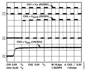
Figure 10. Typical V<sub>DD2</sub> Startup to Output Valid
