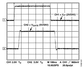
Figure 7. Typical Input to Output Waveform, 2 nF Load, 3.9  $\Omega$  Series Gate Resistor, V<sub>DD1</sub> = 5 V, V<sub>DD2</sub> = 15 V, V<sub>SS2</sub> = 0 V
