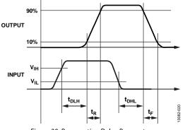
Figure 20. Propagation Delay Parameters
