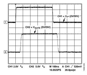
Figure 5. Typical Input to Output Waveform, 2 nF Load, 5.1  $\Omega$  Series Gate Resistor, V<sub>DD1</sub> = 5 V, V<sub>DD2</sub> = 15 V, V<sub>SS2</sub> = 0 V
