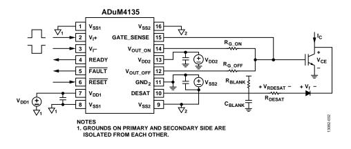
Figure 28. Typical Application Schematic
