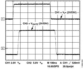
Figure 4. Typical Input to Output Waveform, 2 nF Load, 5.1  $\Omega$  Series Gate Resistor, V<sub>DD1</sub> = +5 V, V<sub>DD2</sub> = +15 V, V<sub>SS2</sub> = -5 V
