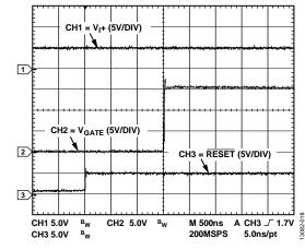
Figure 18. Example RESET to Output Valid
