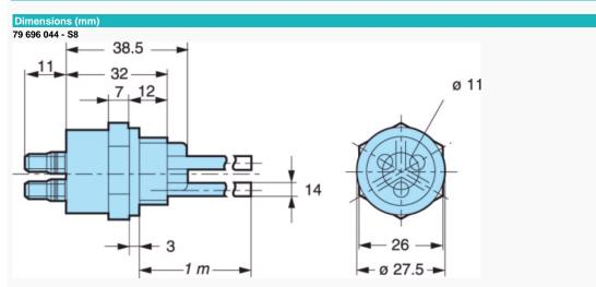
Light and compact 3-probe electrode holder (stainless steel). Electrode holder and 1000 mm probe. Especially recommended for drinks dispensers and for applications where space is limited. Operating temperature : 80 °C Max. pressure : 2 kg/cm 2
