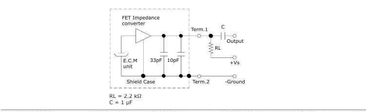
CUI Devices | MODEL: CMC-4012-40P | DESCRIPTION: ELECTRET CONDENSER MICROPHONE
