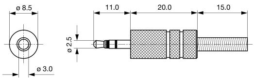
Cable diameter max. 3.0 mm
