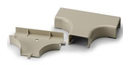
TSRP power rated surface raceway systems have an enhanced "channel and lug" mating design that provides a tighter, more secure fit between raceway lengths and fittings, enabling the system to be UL Listed for power up to 600 volts and meet UL5A and CSA 22.2.
