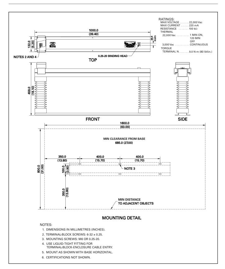
FIG. 15. ER-35KV sensing resistor.
