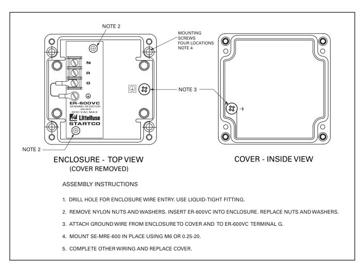
FIG. 10. ER-600VC installed in SE-MRE-600.
