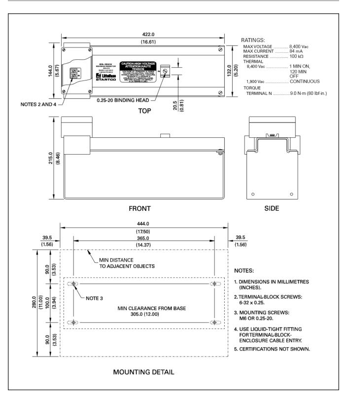
FIG. 13. ER-15KV sensing resistor.
