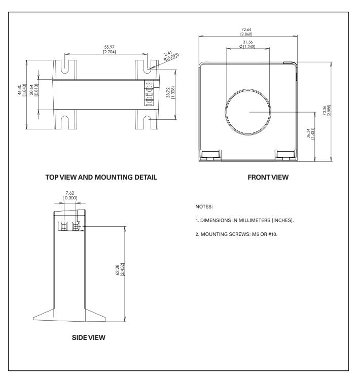
FIG. 17. ELCT5-31 and ELCT30-31 ground-fault current sensors.
