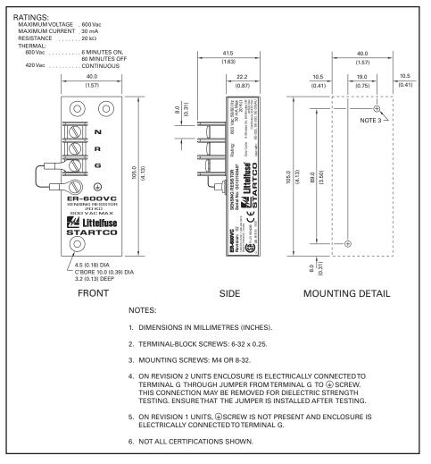
FIG. 8. ER-600VC sensing resistor.
