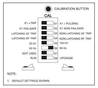
FIG. 1. Configuration switches.
