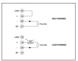
FIG. 2. Analog-output connections.
