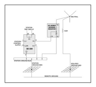
FIG. 20. Simplified isolated-ground connection.
