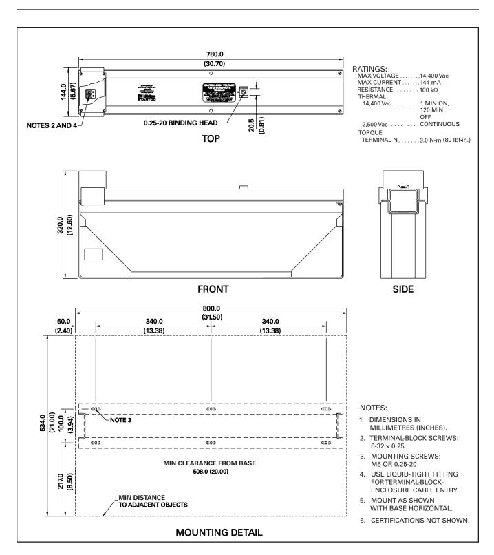
FIG. 14. ER-25KV sensing resistor.
