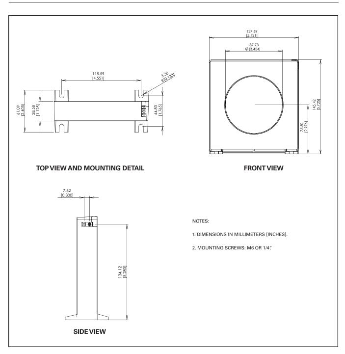
FIG. 16. ELCT5-88 and ELCT30-88 ground-fault current sensors.
