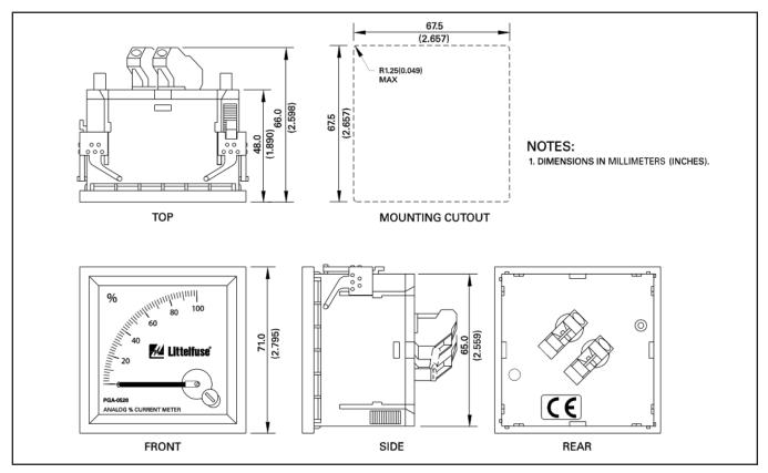
FIG. 19. PGA-0520 analog percent current meter.
