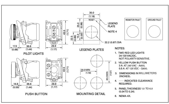
FIG. 18. RK-332 remote indication and reset.
