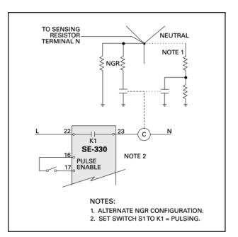
FIG. 21. Simplified pulsing connection.
