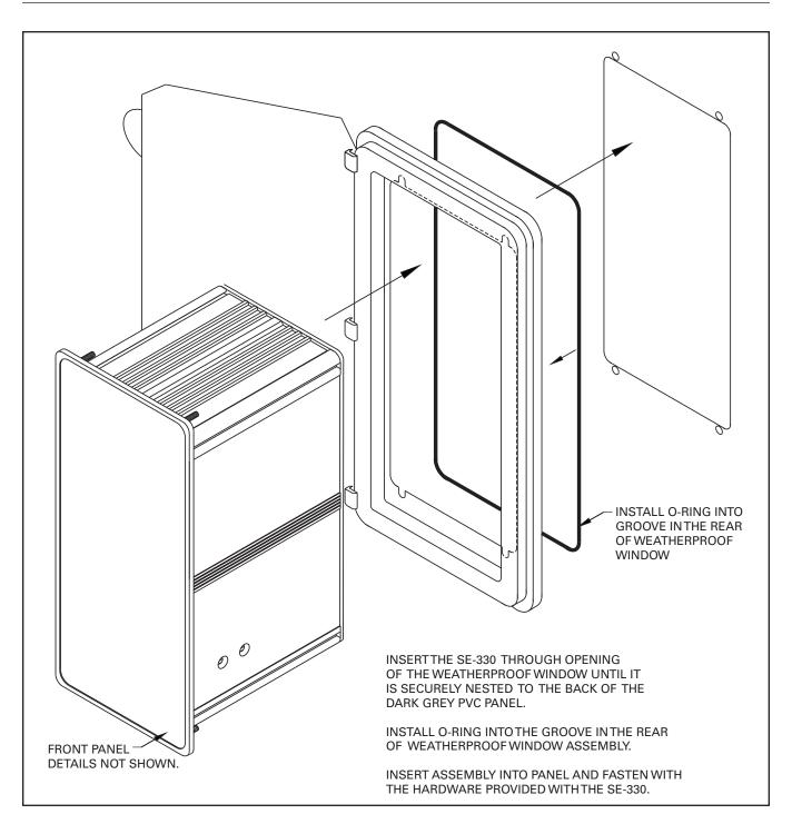
FIG. 7. SE-IP65CVR-G weatherproof cover installation.
