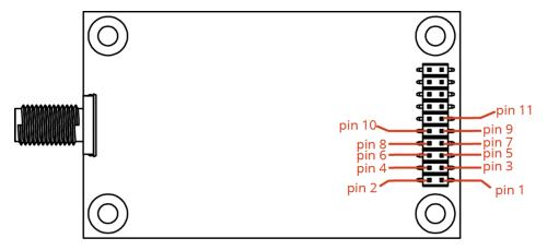
When integrating the module with a Host PC board, leave all lines that you do not use disconnected (floating).
