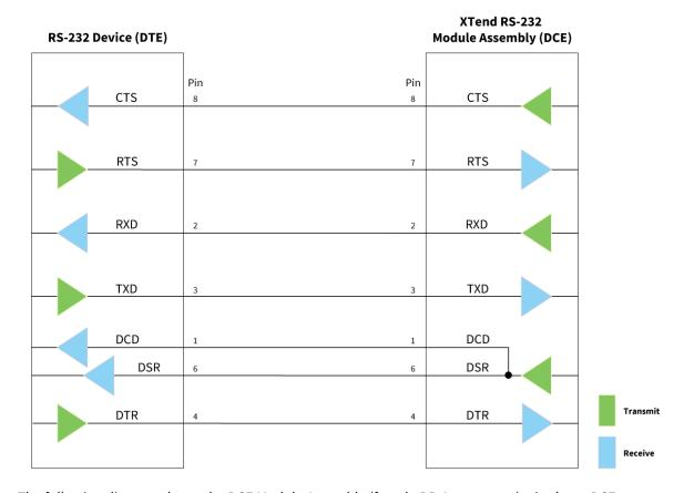
The following diagram shows the DCE Module Assembly (female DB-9 connector) wired to a DCE device (RS-232, male DB-9).
