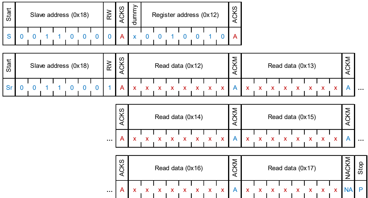
Figure 5: I 2 C multiple read
