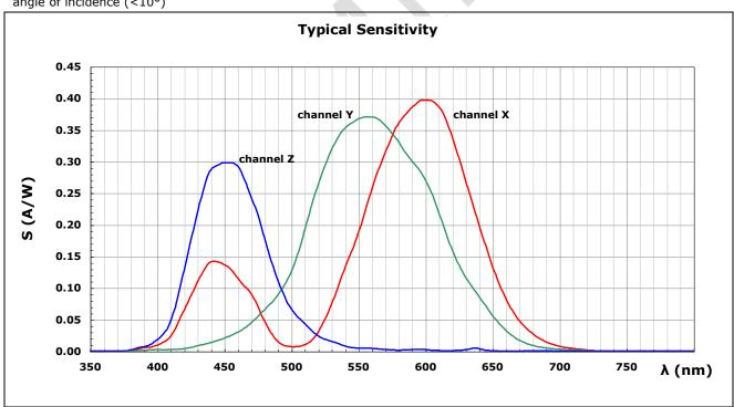
The used JENCOLOR® interference filter technology guarantees high transmission in the band pass range, a very low rest transmission, resistant to aging effects and long-term stable against mechanical and temperature influences during processes.
