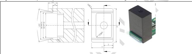
This optional optical cover on the circuit board can be used to limit the angle of aperture / incidence (max.  $\pm 10^{\circ}$  of vertical beam). A special contact surface is used to connect the optical cover to the circuit board, therefore a 2 mm spacing area around the connector and sensor exists. Additionally, two notches are included for equipping a casing.
