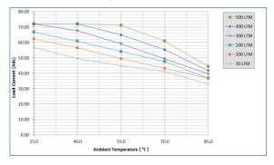
Fig. 5: Available load current vs. ambient air temperature and airflow rates for UIQ48T72033 converter with baseplate equipped with .45" finned heatsink mounted vertically with air flowing from pin 3 to pin 1, MOSFET temperature ≤ 125°C, Vin=48V
