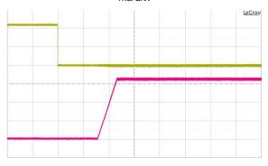
Fig. 11: Output voltage response to load current step change (36 A – 54 A –36 A) at Vin = 48 V. Top trace: output voltage (200 mV/div.). Bottom trace: load current (20 A/div.). Current slew rate: 0.1 A/μs. Co =1 μF ceramic + 10 μF tantalum. Time scale: 200 μs/div.
