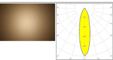
CLU700/701/702 LED  $\mathsf{FWHM}\,/\,\mathsf{FWTM}$ 20.0° / 58.0° Efficiency 79 % Peak intensity 3.1 cd/lm LEDs/each optic Light colour White Required components:
