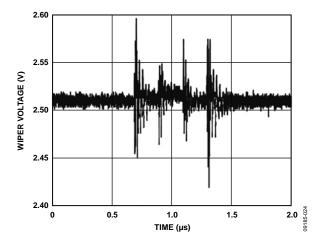
Figure 23. Digital Feedthrough
