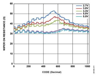
Figure 11. Wiper On Resistance vs. Code
