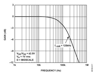
Figure 17. – 3 dB Bandwidth vs. Resistance (See Figure 31)
