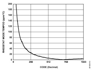
Figure 10. ( $\Delta R_{WB}/R_{WB}$ )/ $\Delta T \times 10^6$  Rheostat Mode Tempco
