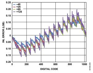
*Figure 5. INL vs. Code, T*<sub>A</sub> = -40°*C,* +25°*C,* +85°*C,* +125°*C Overlay*
