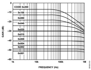
Figure 18. Gain vs. Frequency vs. Code (See Figure 31)
