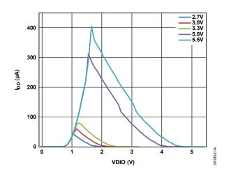
Figure 14. IDD vs. Digital Input Voltage
