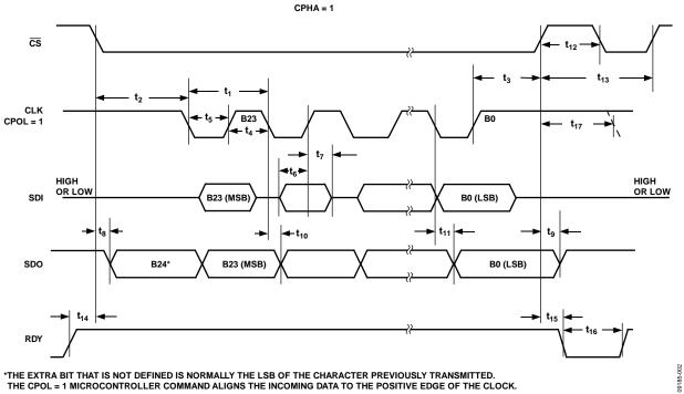
\*THE EXTRA BIT THAT IS NOT DEFINED IS NORMALLY THE LSB OF THE CHARACTER PREVIOUSLY TRANSMITTED. THE CPOL = 1 MICROCONTROLLER COMMAND ALIGNS THE INCOMING DATA TO THE POSITIVE EDGE OF THE CLOCK.
