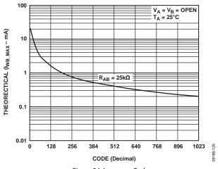
Figure 24. I<sub>WB\_MAX</sub> vs. Code
