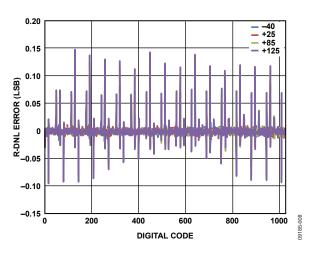
*Figure 8. R-DNL vs. Code, T*<sub>A</sub> = -40°C, +25°C, +85°C, +125°C Overlay
