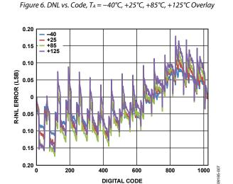
Figure 7. R-INL vs. Code,  $T_A = -40^{\circ}$ C,  $+25^{\circ}$ C,  $+85^{\circ}$ C,  $+125^{\circ}$ C Overlay
