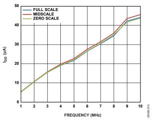
Figure 13. IDD vs. Clock Frequency
