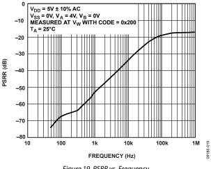
Figure 19. PSRR vs. Frequency
