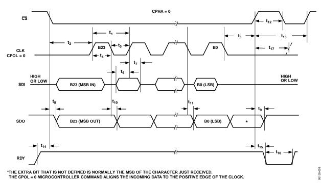
Figure 3. CPHA = 0 Timing Diagram
