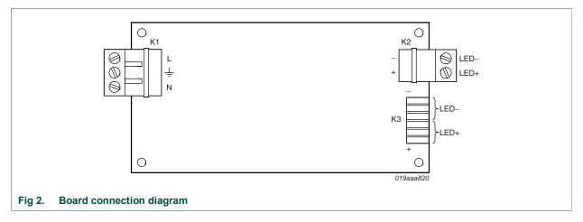
If a galvanic isolated transformer is used, it should be placed between the AC source and the dimmer/demo board. Connect a user defined LED (string) to connector K2 as shown in <u>Figure 2</u>. Note that the anode of the LED (string) is connected to the bottom side of this connector.
