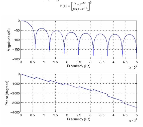
Figure 14. Sinc Filter Response,  $t_S = 8 \ \mu s$
