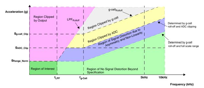
Figure 33. Output Clipping Vs. Frequency
