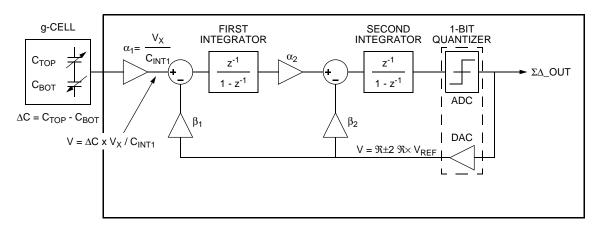
Figure 11.  $\Sigma\Delta$  Converter Block Diagram
