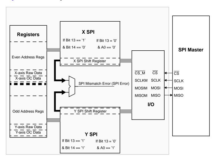
Figure 31 shows an internal diagram of the MMA68xx SPI.
