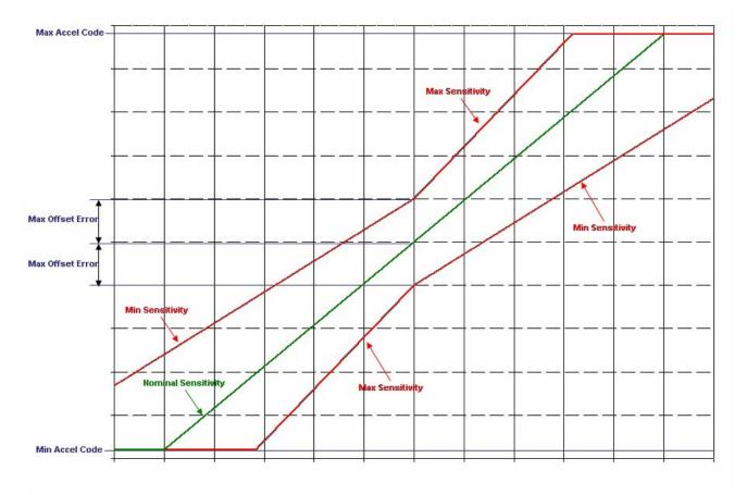
Figure 36. Acceleration Data Output Vs. Acceleration Input
