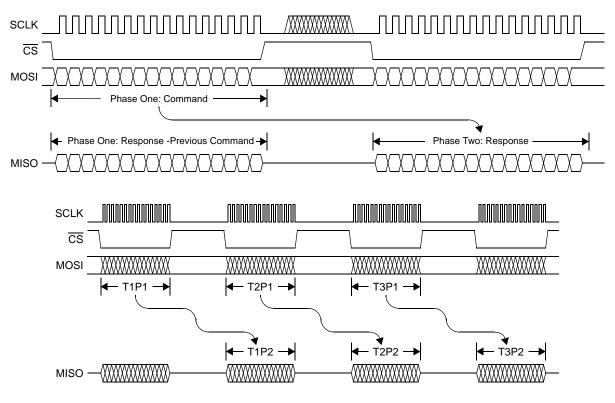
Figure 34. SPI Transfer Detail
