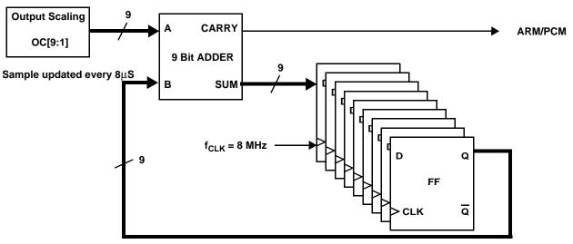
Figure 30. PCM Output Function Block Diagram
