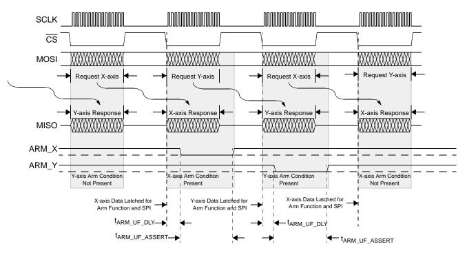
Figure 28. X and Y Axis Arming Conditions, Unfiltered Mode
