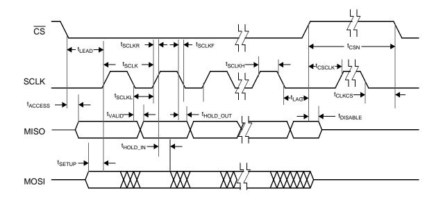
Figure 7. Serial Interface Timing
