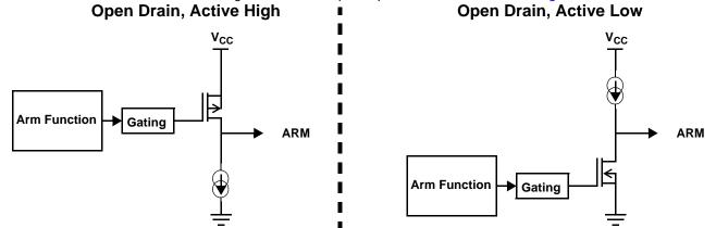
Figure 29. Arming Function - Pin Output Structure
