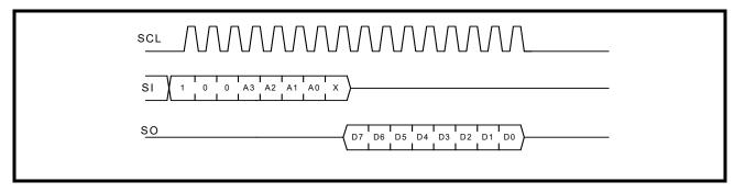
After the last read or write transaction, the SPI master will set the SCL signal back to its idle state (LOW).
