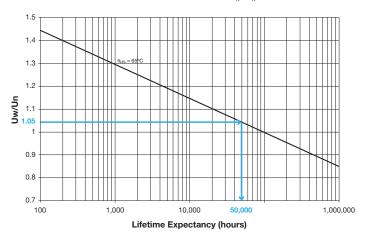
eg: rated voltage 1000V working voltage 1050V  $\rho = 1.05 \Rightarrow$  lifetime 50,000 hours @ 65°C hot spot temperature
