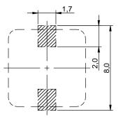
no sensitive traces underneath the component
