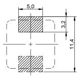
no sensitive traces underneath the component
