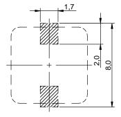
no sensitive traces underneath the component
