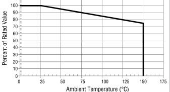
This graph shows the typical device surge current derating versus ambient temperature when subjected to the 8/20  $\mu$ s current waveform per the IEC 61000-4-5 specification. This device is not intended for continuous operation at temperatures above 125 °C.
