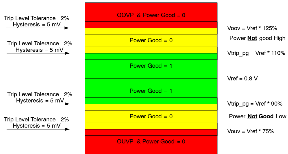
Figure 24. OOV, OUV, and Power Good Window Diagram
