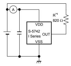
\*1. Resistor (R) is unnecessary for Nch driver + built-in pull-up resistor product.
