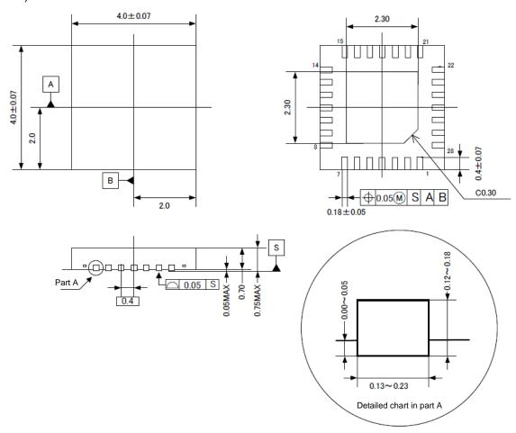
Figure 2 Package outer dimension
