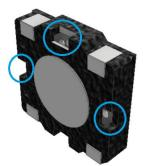
For best frequency response results, fill in these vent holes after reflow or hand soldering to prevent potential cancelation.
