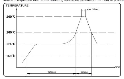
Heat resistant line (Used when heat resistant reliability test is performed)
