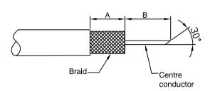
2) Twist the braid in a clockwise direction so that a minimum of 1.0mm dielectric is shown. Make sure to avoid loose or stray strands that could cause short circuits.
