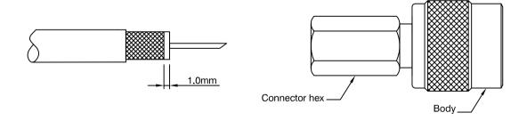
4) Firmly push the cable as far forward as possible and screw the connector hex back end onto the cable in a clockwise direction until it stops.
