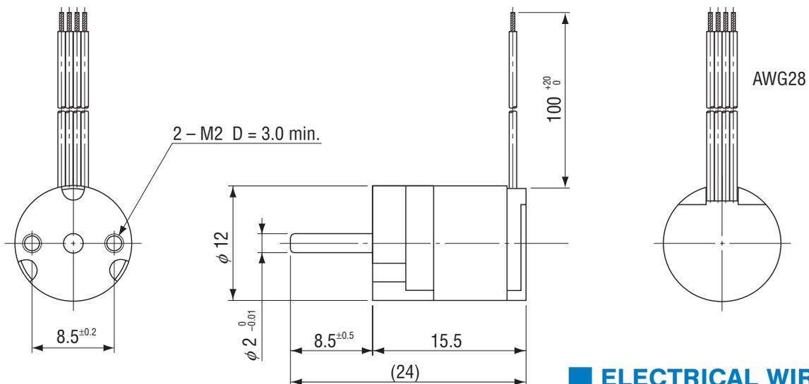
Unless otherwise specified, tolerance : ± 0.4 (Unit : mm)
