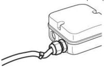
Fig. 2: Fan installed lying flat, cable routed in a U-shaped loop.
