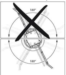
Fig. 3: Cable routing for fans installed upright.
