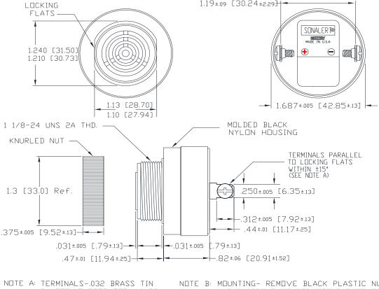
PLATED, TAPPED FOR #6-32 TWO #6-32 NICKEL SCREW. PLATED BRASS SCREWS INCLUDED. WILL ACCEPT 1/4" QUICK CONNECT.
