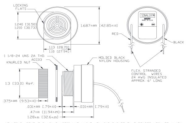
MOUNTING- REMOVE BLACK PLASTIC NUT WHILE LEAVING GASKET ON THREADED NECK OF ALARM. INSERT THREADED NECK THROUGH APPROPRIATE SIZED PANEL HOLE. SCREW NUT BACK ONTO THREADED FRONT SECURING ALARM TO PANEL. MAX RECOMMENDED TORQUE IS 10 IN-LBS.
