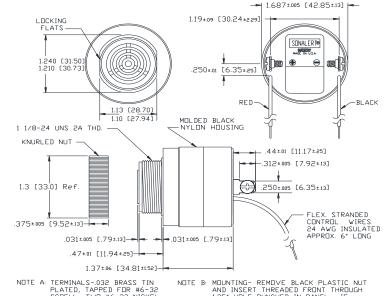
The red and black leads control the several functions. A logic 'Low' is a voltage less than 1/3 of supply voltage. A logic 'High' is a voltage greater than 1/2 supply voltage. A red or black input lead left unconnected is considered an open state.
