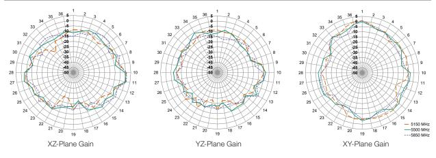
Figure 7. ANT-2/5-HDP-2000-ccc Radiation Patterns
