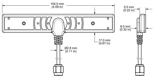
Figure 1. ANT-2/5-HDP-2000 Antenna Dimensions
