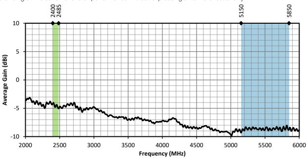
Figure 5. ANT-2/5-HDP-2000 Antenna Average Gain with Frequency Band Highlights
