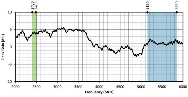
Figure 4. ANT-2/5-HDP-2000 Peak Gain with Frequency Band Highlights
