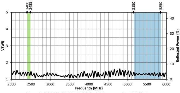
Figure 2. ANT-2/5-HDP-2000 VSWR with Frequency Band Highlights
