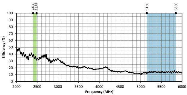
Figure 6. ANT-2/5-HDP-2000 Antenna Radiation Efficiency with Frequency Band Highlights
