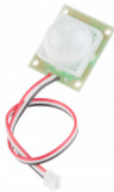
PIR Motion Sensor (JST)
