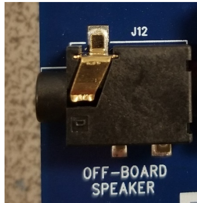
Figure 33 - Off-board Speaker Connector
