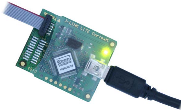
Figure 44 - Segger J-Link Lite Cortex M 10-pin Adapter
