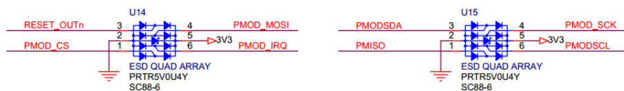
Figure 42 - Pmod Connector ESD Protection Schematic
