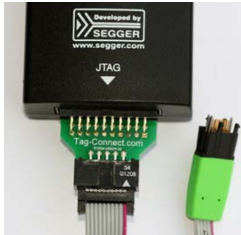
Figure 48 - Tag Connect Header & Connector
