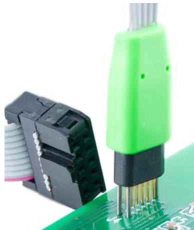
Figure 49 - Tag Connect Header inserted into PCB
