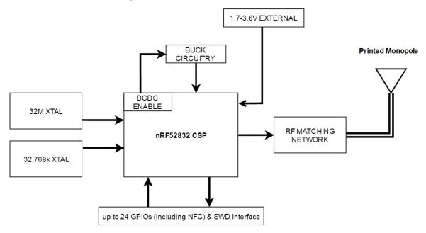
Figure 5: D52MD2M8IA, D52MPMM8IA Models Module Block Diagram
