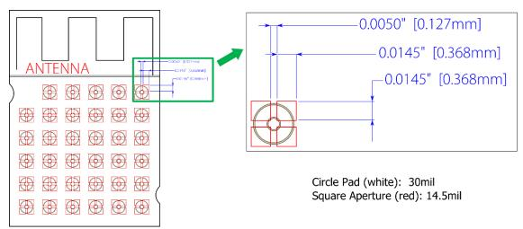
Figure 16: D52M M8 Solder Stencil
