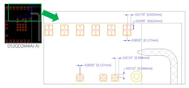
Figure 15: D52Q M4 Solder Stencil
