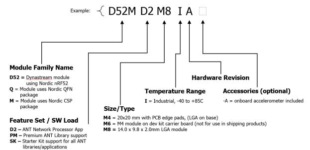
Figure 1: D52 Module Series Nomenclature
