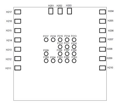
Figure 6: D52Q M4 (20mm x 20mm) Bottom View
