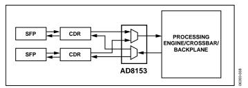
Figure 35. Line Interface Redundancy Application
