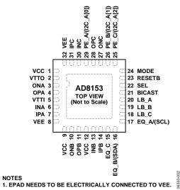
Figure 3. Pin Configuration
