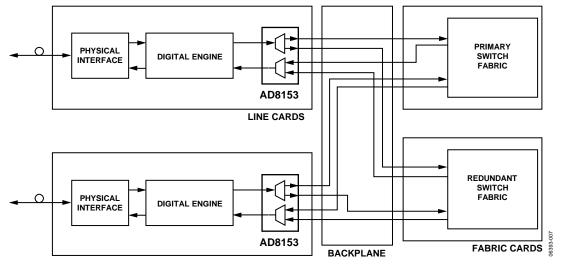
Figure 34. Switch Redundancy Application
