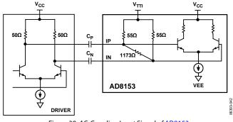
Figure 39. AC-Coupling Input Signal of AD8153
