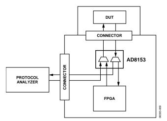
Figure 36. Test Equipment Application
