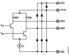
Figure 38. Transmitter Simplified Diagram
