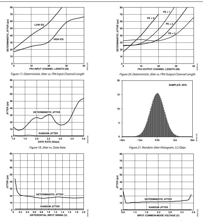
Figure 19. Jitter vs. Differential Input Swing
