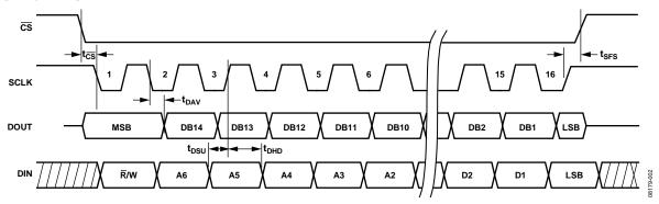
Figure 2. SPI Timing and Sequence
