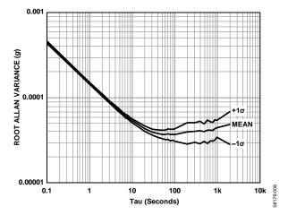
Figure 8. Accelerometer Allan Variance
