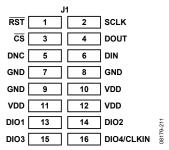
Figure 17. J1 Pin Assignments for the ADIS16IMU2/PCBZ
