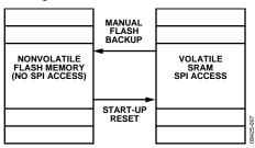
Figure 7. SRAM and Flash Memory Diagram
