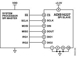
Figure 8. Electrical Hook-Up Diagram
