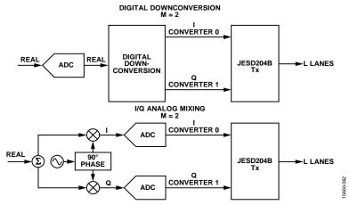
Figure 91. I/Q Transport Layer Mapping
