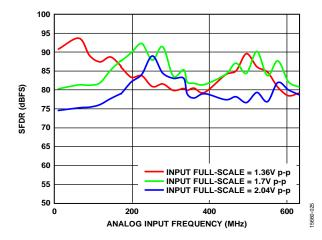
Figure 53. SFDR vs. Analog Input Frequency with Different Analog Input Full-Scale Values (A<sub>IN</sub> < 650 MHz)
