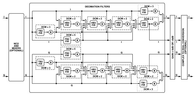
FIR = FINITE IMPULSE RESPONSE FILTER DCM = DECIMATION
