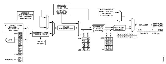
Figure 142. ADC Output Datapath Showing Data Framing
