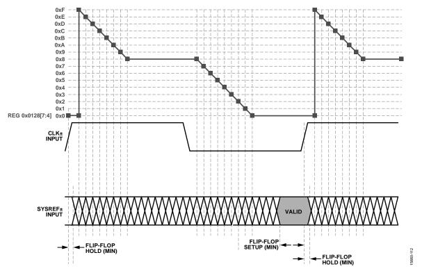
Figure 141. SYSREF± Hold Detector
