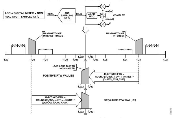
Figure 99. DDC NCO Frequency Tuning Word Selection—Real Inputs
