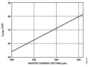
Figure 32. I<sub>AVDD3</sub> vs. Buffer Control 1 Setting in Register 0x1A4C
