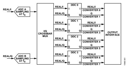
Figure 90. DDCs and Virtual Converter Mapping
