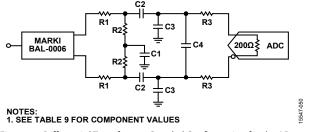
Figure 69. Differential Transformer-Coupled Configuration for the AD9695
