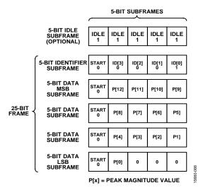
Figure 117. SPORT over JESD204B Signal Monitor Frame Data
