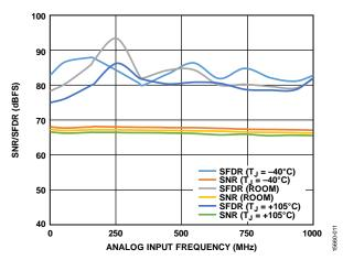
Figure 38. SNR/SFDR vs. Analog Input Frequency (f<sub>IN</sub>) at Minimum, Room, and Maximum Temperatures
