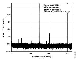
Figure 10. Single-Tone FFT with  $f_{IN} = 1002.3 \text{ MHz}$
