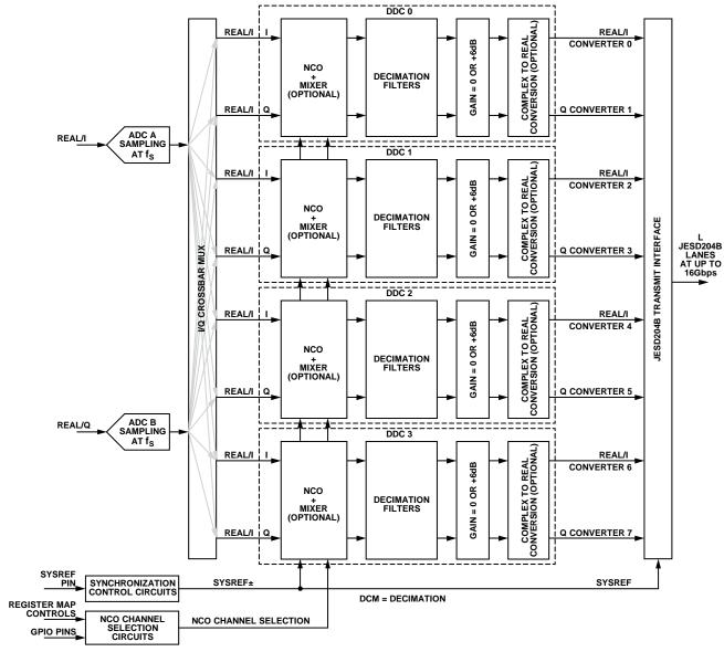
Figure 97. DDC Detailed Block Diagram
