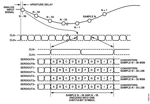
Figure 2. Data Output Timing Diagram
