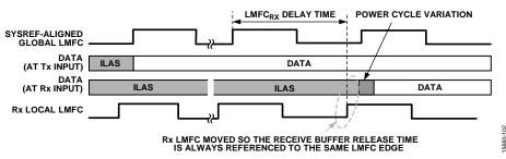
Figure 131. Adjusting the JESD204B Rx LMFC in the Logic Device
