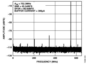
Figure 9. Single-Tone FFT with  $f_{IN} = 752.3$  MHz
