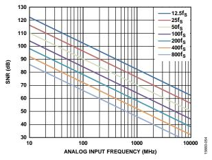
Figure 83. Ideal SNR vs. Input Frequency and Jitter
