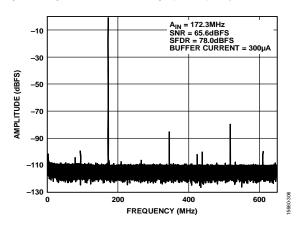
Figure 7. Single-Tone FFT with Analog Input Frequency  $(f_{IN}) = 172.3 \text{ MHz}$
