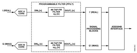
Figure 92. Real 48-Tap Filter Configuration
