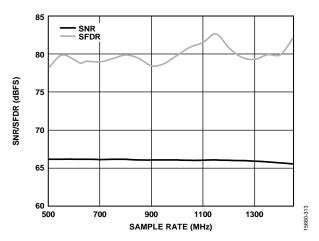
Figure 14. SNR/SFDR vs. Sample Rate,  $f_{IN} = 172.3 \text{ MHz}$
