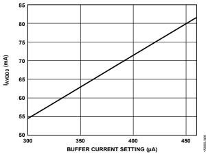
Figure 72. AVDD3 Current (I<sub>AVDD3</sub>) vs. Buffer Current Setting (Buffer Control 1 Setting in Register 0x1A4C and Buffer Control 2 Setting in Register 0x1A4D)
