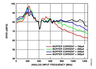
Figure 50. SFDR vs. Analog Input Frequency with Different Buffer Current Settings (A<sub>IN</sub> < 1250 MHz)
