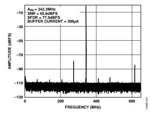
Figure 8. Single-Tone FFT with  $f_{IN} = 342.3 \text{ MHz}$
