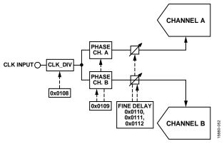
Figure 81. Clock Divider Phase and Delay Controls
