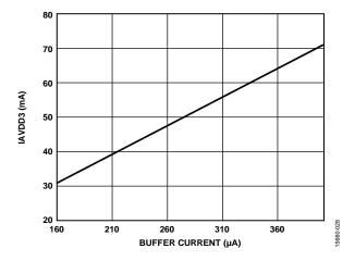
Figure 56. I<sub>AVDD3</sub> vs. Buffer Control 1 Setting in Register 0x1A4C
