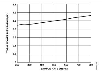
Figure 48. Total Power Dissipation vs. Sample Rate (fs)
