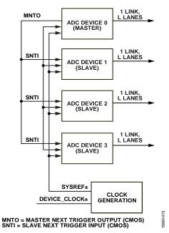
Figure 104. System Using Master/Slave Synchronization Triggering
