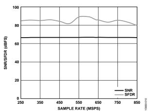
Figure 37. SNR/SFDR vs. Sample Rate,  $f_{IN} = 172.3 \text{ MHz}$
