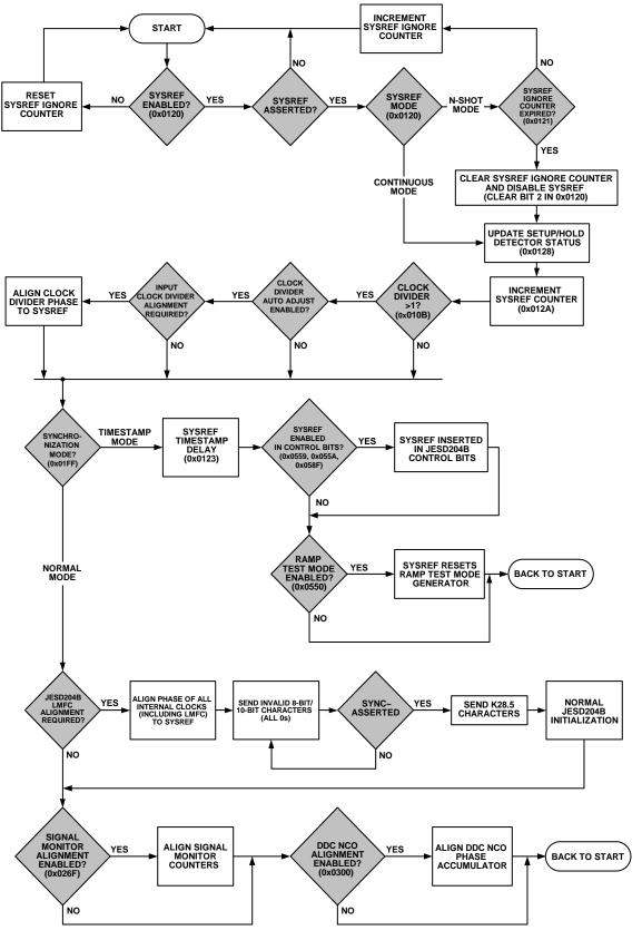
Figure 133. SYSREF± Capture Scenarios and Multichip Synchronization
