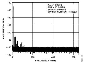
Figure 6. Single-Tone FFT with Analog Input Frequency  $(f_{IN}) = 10.3 \text{ MHz}$
