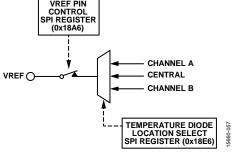
Figure 86. Register Controls to Output Temperature Diode Voltage on the VREF Pin
