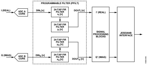
Figure 94. Real, Two Cascaded, 24-Tap Filter Configuration
