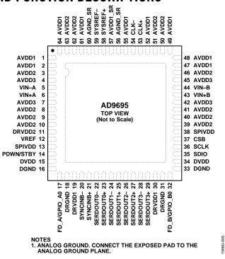
Figure 5. Pin Configuration (Top View)
