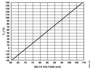
Figure 88. Junction Temperature (T<sub>J</sub>) vs. Delta Voltage (ΔV)
