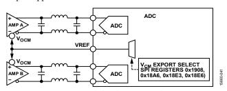
Figure 70. DC-Coupled Application Using the AD9695
