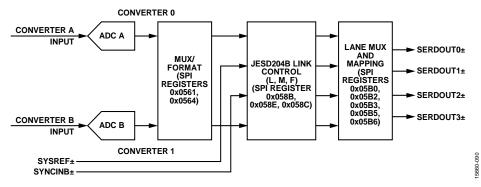
Figure 119. Transmit Link Simplified Block Diagram Showing Full Bandwidth Mode (Register 0x200 = 0x00)
