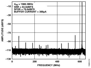
Figure 13. Single-Tone FFT with  $f_{IN} = 1980.3 \text{ MHz}$
