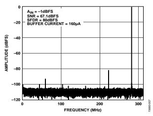
Figure 34. Single-Tone FFT with  $f_{IN} = 340 \text{ MHz}$
