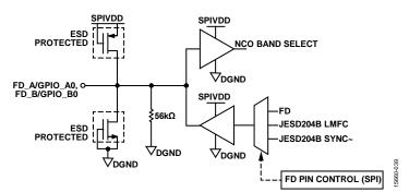
Figure 67. FD\_A/GPIO\_A0 and FD\_B/GPIO\_B0
