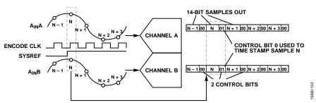
Figure 132. AD9695 Timestamping—CS = 2 (Register 0x058F, Bits[7:6] = 2), Control Bit 1 is SYSREF± (Register 0x0559, Bits[6:4] = 5)
