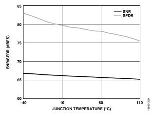
Figure 21. SNR/SFDR vs. Junction Temperature,  $f_{IN} = 172.3 \text{ MHz}$
