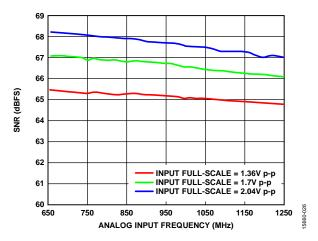
Figure 54. SNR vs. Analog Input Frequency with Different Analog Input Full-Scale Values (A<sub>IN</sub> > 650 MHz)
