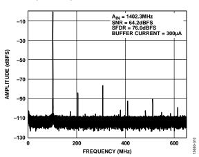
Figure 11. Single-Tone FFT with  $f_{IN} = 1402.3 \text{ MHz}$
