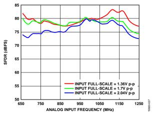
Figure 55. SFDR vs. Analog Input Frequency with Different Analog Input Full-Scale Values (A<sub>IN</sub> > 650 MHz)
