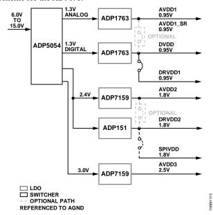
Figure 143. High Efficiency, Low Noise Power Solution for the AD9695
