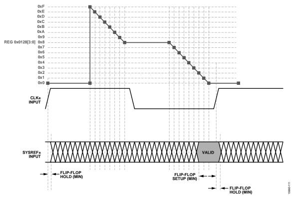
Figure 140. SYSREF± Setup Detector
