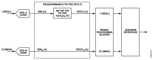
Figure 93. Real 96-Tap Filter Configuration
