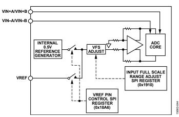
Figure 73. Internal Reference Configuration and Controls
