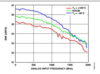
Figure 15. SNR vs. Analog Input Frequency (f<sub>IN</sub>) at Minimum, Room, and Maximum Temperatures
