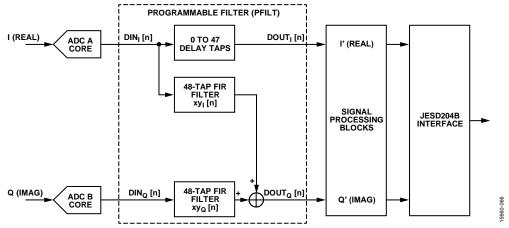
Figure 95. 48-Tap Half Complex Filter Configuration
