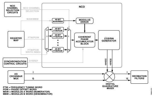
Figure 101. NCO + Mixer Block Diagram
