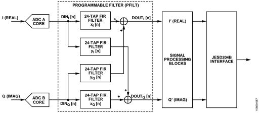
Figure 96. 24-Tap Full Complex Filter Configuration.
