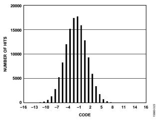
Figure 24. Input Referred Noise Histogram
