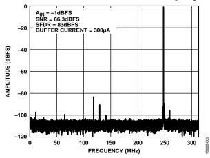
Figure 36. Single-Tone FFT with  $f_{IN} = 1000 \text{ MHz}$
