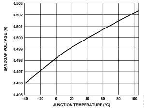
Figure 75. Typical V<sub>REF</sub> Drift
