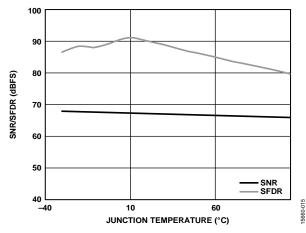
Figure 42. SNR/SFDR vs. Junction Temperature,  $f_{IN} = 172.3 \text{ MHz}$
