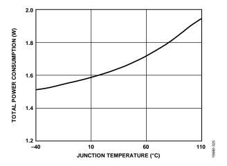
Figure 26. Total Power Dissipation vs. Junction Temperature
