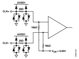
Figure 58. Clock Inputs
