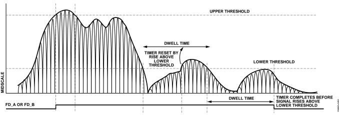
Figure 89. Threshold Settings for FD\_A and FD\_B Signals
