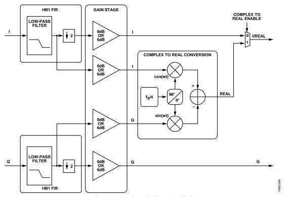
Figure 114. Complex to Real Conversion Block
