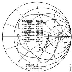
Figure 68. AD9695 Different Input Return Loss
