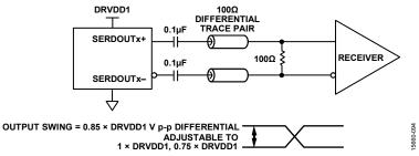
Figure 123. AC-Coupled Digital Output Termination Example
