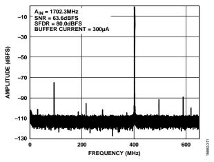
Figure 12. Single-Tone FFT with  $f_{IN} = 1702.3 \text{ MHz}$
