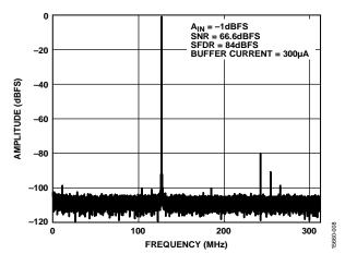
Figure 35. Single-Tone FFT with  $f_{\rm IN}$  =750 MHz
