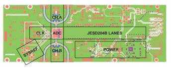
Figure 145. Recommended PCB Layout for the AD9695
