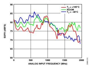
Figure 16. SFDR vs. Analog Input Frequency (f<sub>IN</sub>) at Minimum, Room, and Maximum Temperatures
