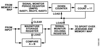
Figure 115. Signal Monitor Block
