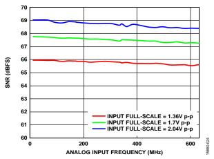
Figure 52. SNR vs. Analog Input Frequency with Different Analog Input Full-Scale Values ( $A_{\rm IN}$  < 650 MHz)
