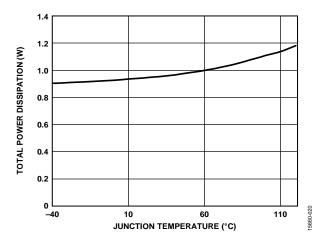
Figure 47. Total Power Dissipation vs. Junction Temperature
