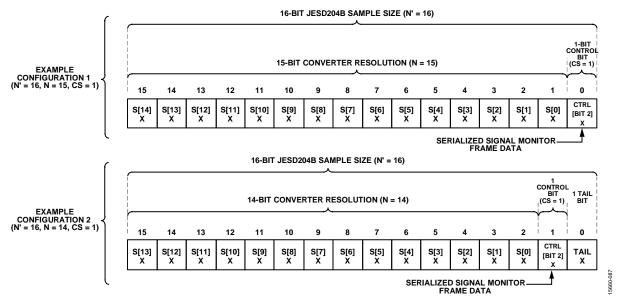
Figure 116. Signal Monitor Control Bit Locations
