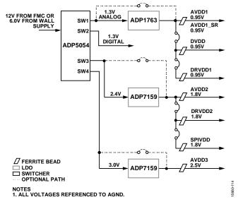
Figure 144. Simplified Power Solution for the AD9695
