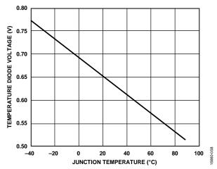
Figure 87. Typical Voltage Response of the 1× Temperature Diode
