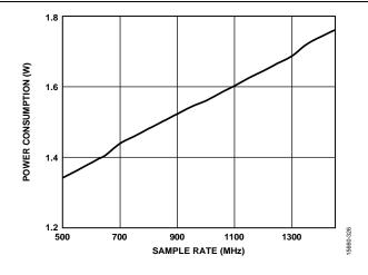
Figure 27. Total Power Dissipation vs. Sample Rate (fs)
