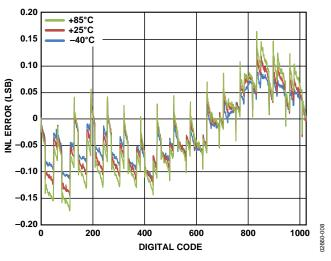
Figure 6. R-INL vs. Code,  $T_A = -40$ °C, +25°C, +85°C Overlay,  $R_{AB} = 25$  k $\Omega$
