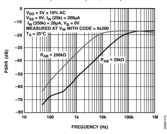
Figure 13. PSRR vs. Frequency
