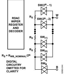
Figure 32. Equivalent RDAC Structure
