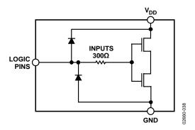
Figure 26. Equivalent ESD Digital Input Protection
