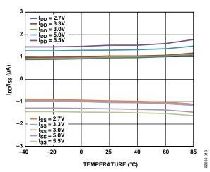
Figure 10.  $I_{DD}$  vs. Temperature,  $R_{AB} = 25 \text{ k}\Omega$
