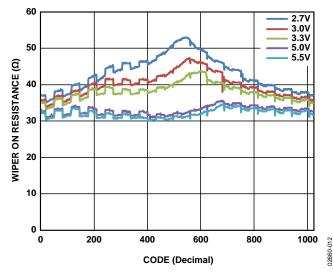
Figure 9. Wiper On Resistance vs. Code
