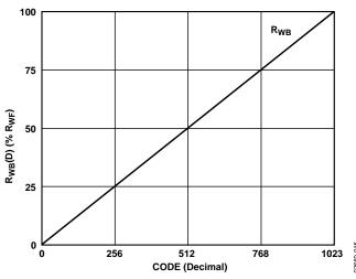
Figure 33. R<sub>WB</sub>(D) vs. Decimal Code
