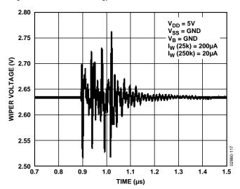
Figure 17. Digital Feedthrough
