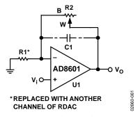
Figure 42. Linear Gain Control with Tracking Resistance Tolerance, Drift, and Temperature Coefficient
