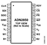
Figure 4. 16-Lead TSSOP Pin Configuration
