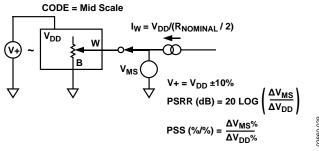
Figure 22. Power Supply Sensitivity (PSS, PSRR)
