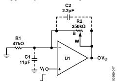
Figure 34. Typical Noninverting Gain Amplifier
