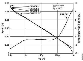
Figure 39.  $V_2 - V_1$  Error vs. Input Current.
