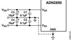
Figure 30. Power Supply Bypassing
