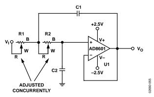
Figure 35. Sallen-Key Low-Pass Filter
