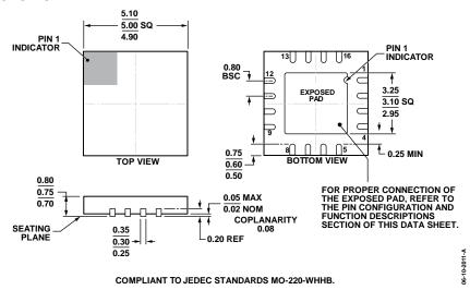
Figure 44. 16-Lead Lead Frame Chip Scale Package [LFCSP] 5 mm × 5 mm Body and 0.75 mm Package Height (CP-16-31) Dimensions shown in millimeters
