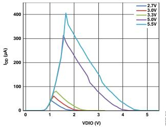
Figure 12. IDD vs Digital Input Voltage
