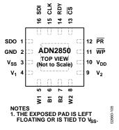
Figure 5. 16-Lead LFCSP Pin Configuration
