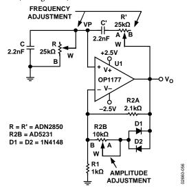
Figure 36. Programmable Oscillator with Amplitude Control
