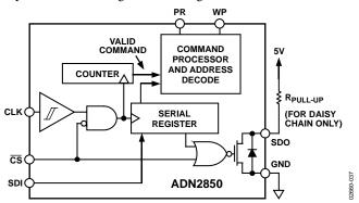
Figure 25. Equivalent Digital Input and Output Logic
