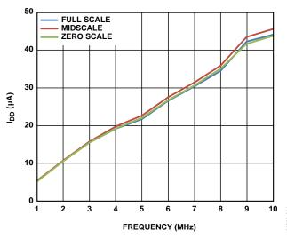
Figure 11. IDD vs. Clock Frequency
