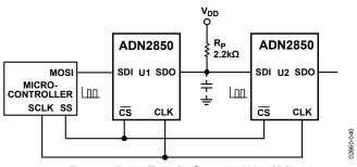
Figure 28. Daisy-Chain Configuration Using SDO
