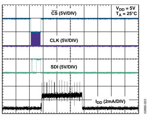
Figure 18. IDD vs. Time when Storing Data to EEMEM
