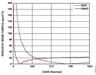
Figure 8.  $(\Delta R_{WB}/R_{WB})/\Delta T \times 10^6$  Rheostat Mode Tempco
