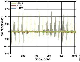
Figure 7. R-DNL vs. Code,  $T_A = -40$ °C, +25°C, +85°C Overlay,  $R_{AB} = 25$  k $\Omega$
