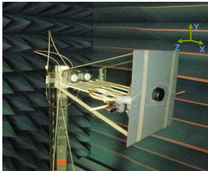
Figure 2. Peak gain, efficiency and radiation pattern measurements.
