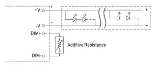
"DO NOT connect "DIM- to -V"
