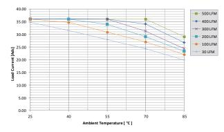
Fig. 2: Power derating vs. ambient air temperature and airflow rates for UIE48T36033 converter w/o baseplate Fig. 3: Available load current vs. ambient air temperature and airflow rates for UIE48T36033 converter w/o baseplate mounted vertically with air flowing from pin 3 to pin 1, MOSFET temperature ≤ 125°C, Vin=24V
