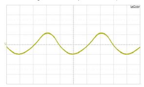
Fig. 16: Input reflected ripple current, is (20 mA/div.), measured through 10 μH at the source at full rated load current and Vin =48 V. Refer to Fig. 14 for test setup. Time scale: 1 μs/div.
