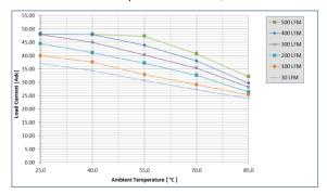
Fig. 5: Available load current vs. ambient air temperature and airflow rates for UIQ48T48050 converter with baseplate equipped with .45" finned heatsink mounted vertically with air flowing from pin 3 to pin 1, MOSFET temperature ≤ 125°C, Vin=48V
