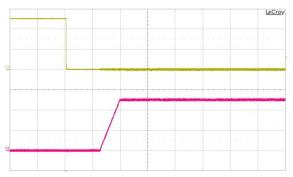
Fig. 11: Output voltage response to load current step change (24A – 36A –24A) at Vin = 48 V. Top trace: output voltage(200mV/div.). Bottom trace: load current (20 A/div.). Current slew rate: 0.1 A/μs. Co =1μF ceramic + 10μF tantalum. Time scale: 200μs/div.
