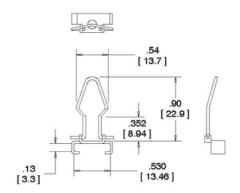
Plastic Connector Mounted to Front of Panel
