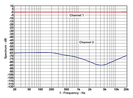
Figure 12. Channel Separation, BTL
