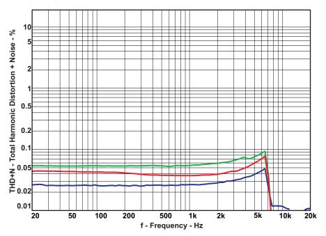
Figure 6. THD+N vs Frequency, BTL  $-8 \Omega$
