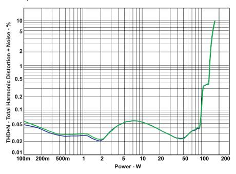
Figure 4. THD+N vs Power, BTL  $-8~\Omega$
