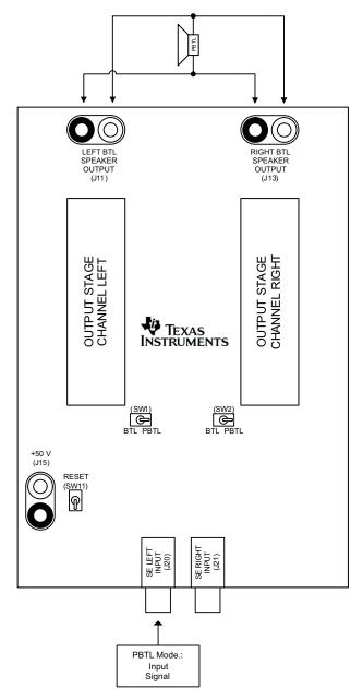
Figure 3. Output Configuration BTL and PBTL
