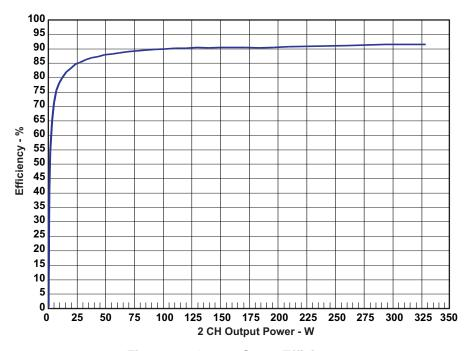
Figure 19. Output Stage Efficiency
