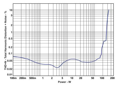
Figure 5. THD+N vs Power, PBTL – 4  $\Omega$
