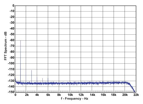
Figure 10. FFT Spectrum With -60-dBFS Tone, PBTL
