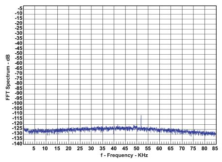
Spurious tone at 52 kHz has its origin from the TL2575 switching voltage regulator.
