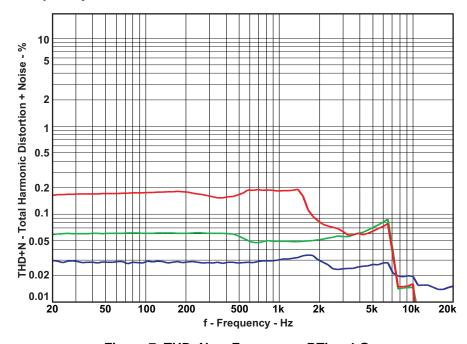
Figure 7. THD+N vs Frequency, BTL – 4  $\Omega$
