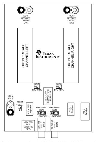
Figure 2. Physical Structure for the TAS5615PHD2EVM (Approximate Layout)
