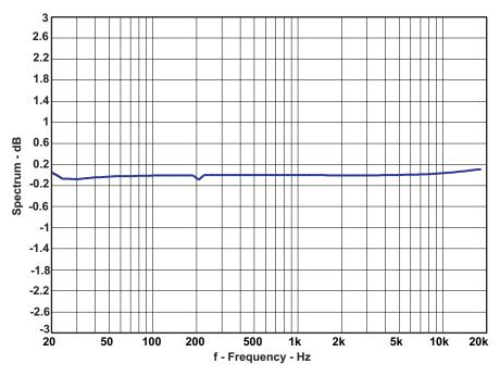
Figure 14. Frequency Response, PBTL
