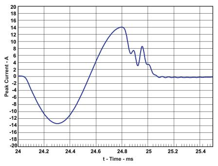
Figure 16. High-Current Protection, PBTL
