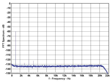
Figure 8. FFT Spectrum with -60-dBFS Tone, BTL
