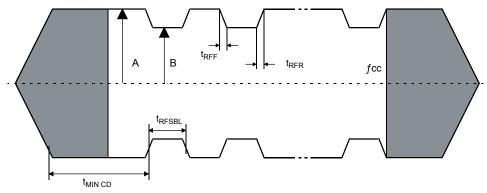
FRAME Transmission between the reader and the contactless device
