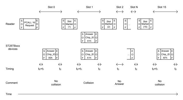
Figure 15. Description of a possible anticollision sequence
